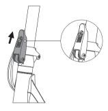
①Slide the sliding buckle on the folding wrench up,
