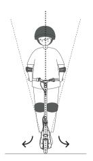
6.When you need to stop, release the acceleration handle to reduce speed, squeeze and brake the handlebar. Lay down the foot support and let the vehicle lean slightly in the foot support direction so that the foot support touches the ground, and the vehicle can be stabilized.
